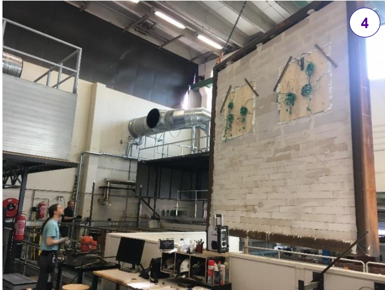
Preparation of dovetail specimens for fire resistance test at Tampere University Fire Laboratory (4) moving the wall to the furnace (5) connecting sensors
