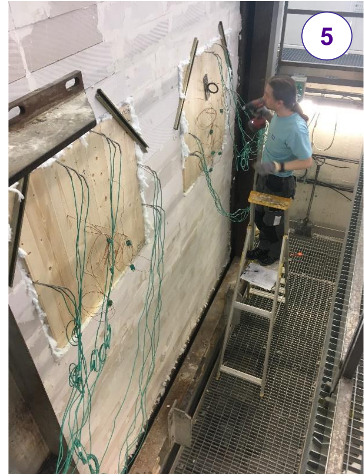
Preparation of dovetail specimens for fire resistance test at Tampere University Fire Laboratory (4) moving the wall to the furnace (5) connecting sensors
