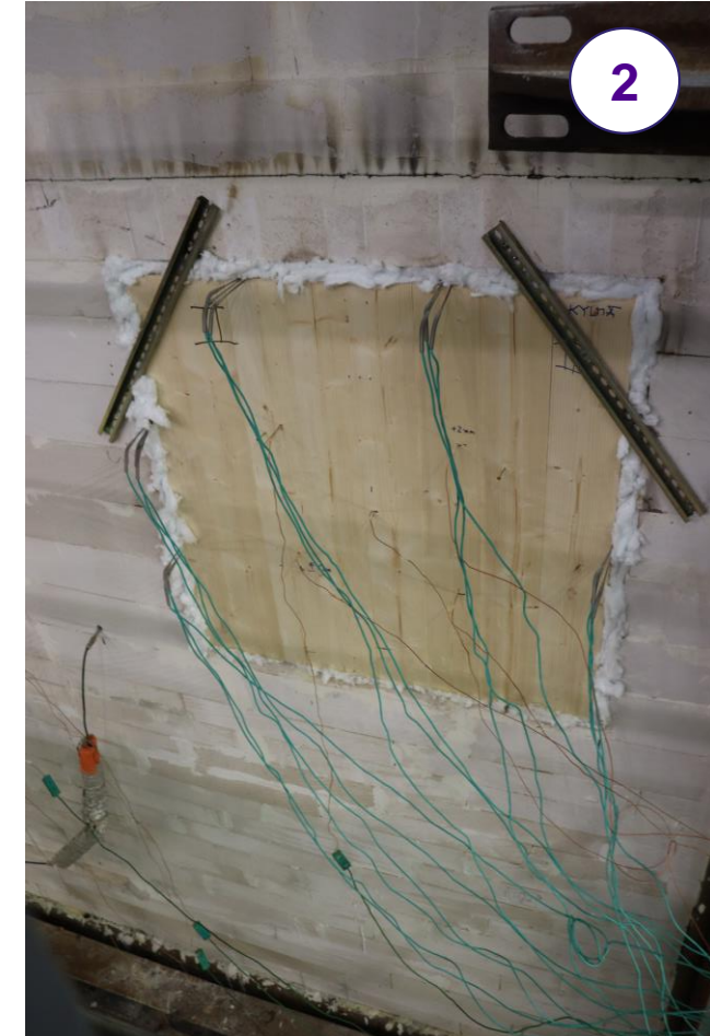
Preparation of CLT specimens for fire resistance test at Tampere University Fire Laboratory (1) drilling & thermocouple insertion (2) mounting on the supporting construction
