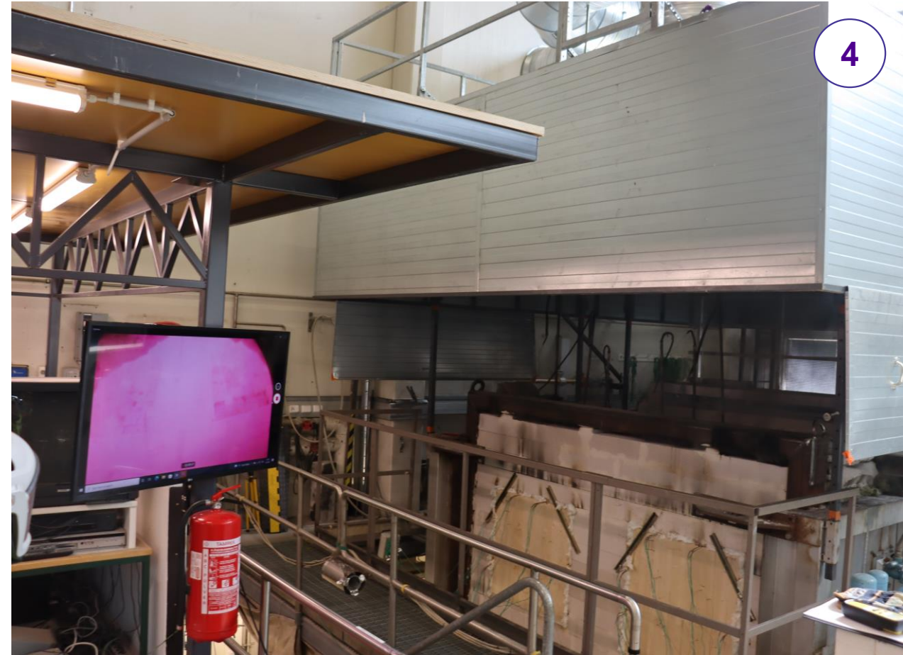
(3) moving the wall to the furnace & connecting sensors (4) BURNING
