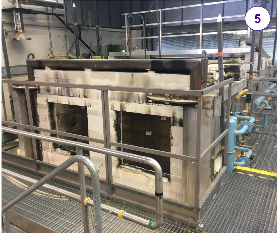
(5) disassembly of test pieces and removal of sensors (6) cutting specimens
