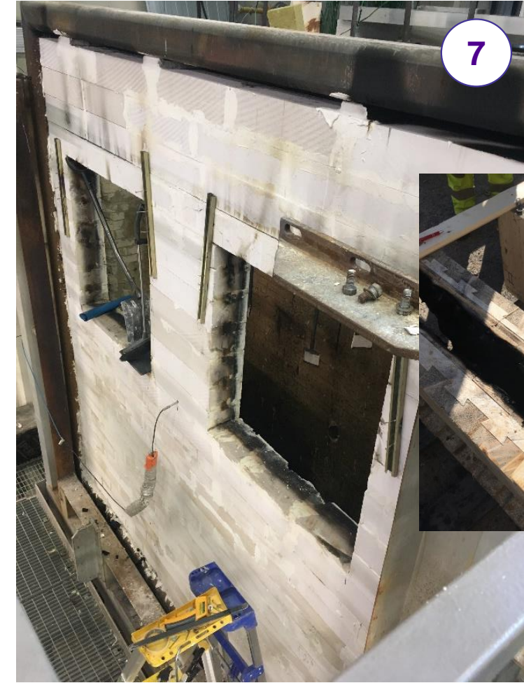
(6) BURNING (7) disassembly of test pieces and removal of sensors (8) cutting specimens
