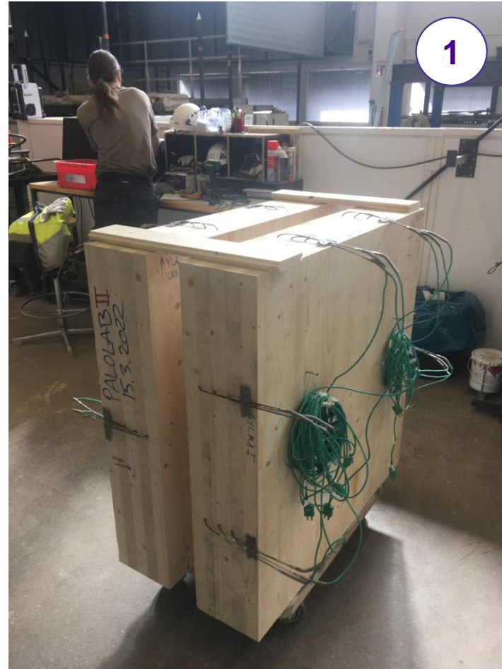
Preparation of CLT specimens for fire resistance test at Tampere University Fire Laboratory (1) drilling & thermocouple insertion (2) mounting on the supporting construction
