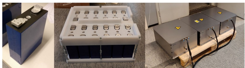
Fig. 5 LFP cell (left), a mechanically supported module consisting of 12 cells in series (middle), and three modules enclosed in separate steel boxes (right)
